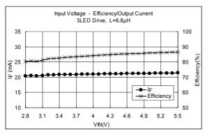
Input Voltage - Efficiency/Output Current
